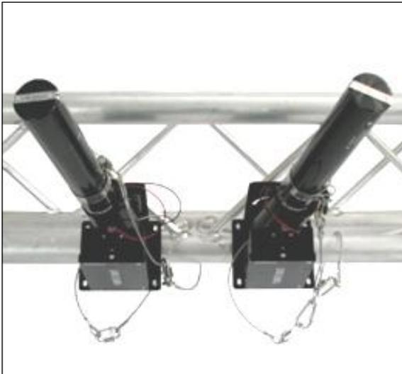
If you want to use the Power Shot while mounted in a truss system, then attach 2 certified truss clamps (MFX3103) to the underside of the Power Shot. Next, place the Power Shot on the required place in the truss system and firmly turn the clamp.
