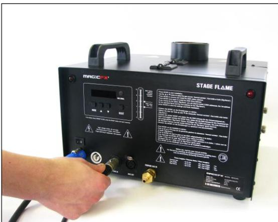
Connect a 3-pole DMX cable to the Stage Flame.
