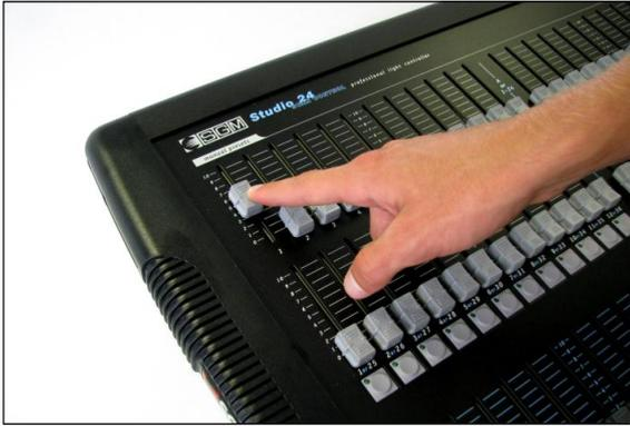
After you have used the Stage Flame, you must set it to safety mode again. You put the Stage Flame in safety mode by sliding shut the safety channel or setting it to a value outside the 40% to 60% range.
