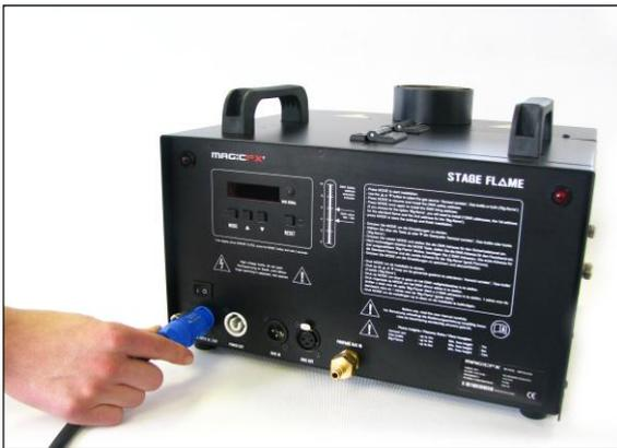
Turn off the Stage Flame power button and disconnect the powerCON cable and DMX plugs.
