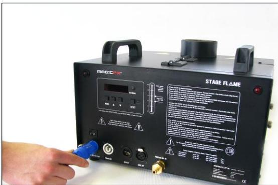
Ensure the Power button is set to “off”. Connect the power cable. The Stage Flame runs on 230V~ 50/60Hz. You will need a powerCON plug to be able to connect the Stage Flame to the power supply. The Stage Flame is delivered with a powerCON looping cable. It can be used to connect multiple Stage Flame devices up to the same power source.
