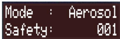
Press MENU again to save your selection. Now the DMX addresses need to be entered. First, the “safety” address needs to be set. You select the channel by using the UP and DOWN buttons. Press the MENU button to save the setting.
