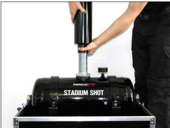
Unscrew the shot pipe from the screw thread integrated in the tank and store these in their flight case holder.
