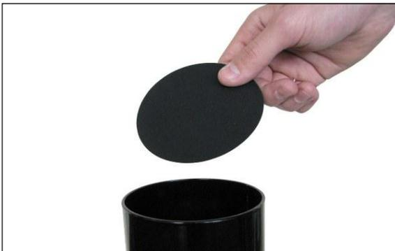
**Take a carton lifting core and lower this to the bottom of the shooting tube to close off the hole.**
