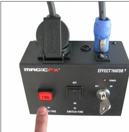
Press the switch to the on (ON) position to enable the Stadium Shot to shoot. Immediately after the shot press the switch again to the off (OFF) position.
