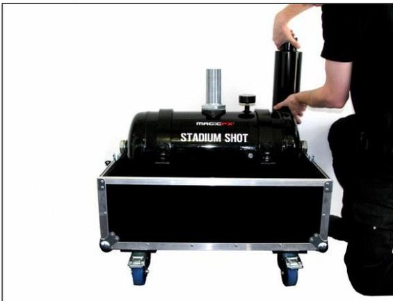
Take the filled shot pipe from the holder in the flight case.
