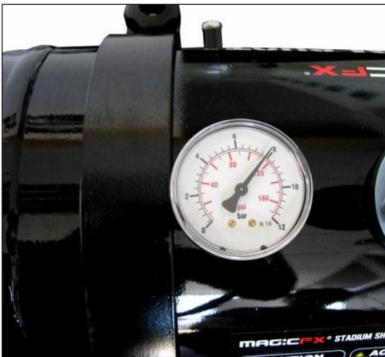
**Activate the compressor and fill the tank until the compressor turns off or the manometer indicates that the pressure in the tank is 8 bar.**
