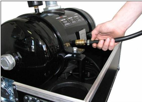
**Take a compressor (with a maximum pressure output of 8 bar), which meets the safety requirements and standards concerned, and connect the hose to the quick-connect coupling of the tank and the quick-connect coupling of the compressor.**
