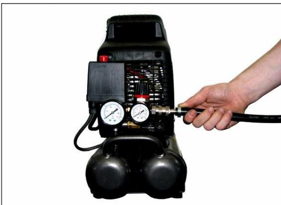
Disconnect the air hose and remove the compressor.
