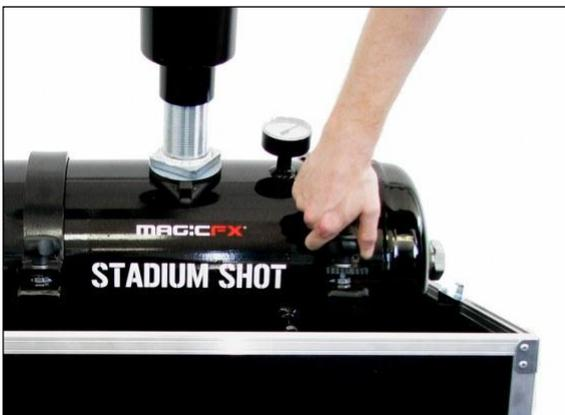
Secure the tank by turning the two fastening buttons. Make sure to twist these buttons properly until the tank is entirely secured.
