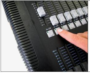
Press the flash button for the selected "fire" channel on the DMX controller. A flame should now be emitted from the Stage Flame.
