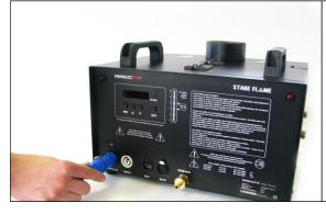
Ensure the Power button is set to "off". Connect the power cable. The Stage Flame runs on 230V~ 50/60Hz. You will need a powerCON plug to be able to connect the Stage Flame to the power supply. The Stage Flame is delivered with a powerCON looping cable. it You can use the powerCON looping cable to connect multiple Stage Flame devices up to the same power source.
