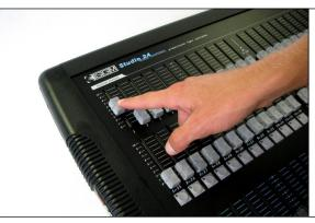
After you have used the Stage Flame, you must set it to safety mode again. You put the Stage Flame in safety mode by sliding shut the safety channel or setting it to a value outside the 40% to 60% range.
